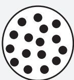
Microcapsule with solid microdomains/nanodomains
